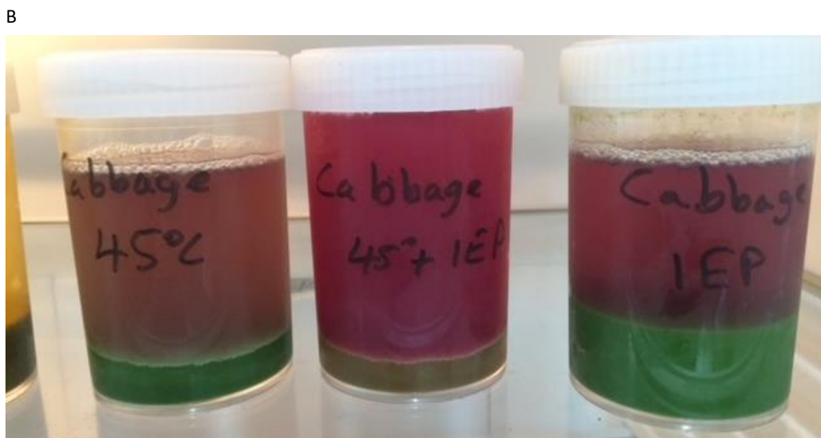
Figure 7. A red and green cabbage juice blend after protein precipitation was induced by heat and/or acidification (IEP).
