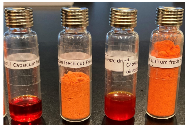
Figure 4: \beta -Carotene oil extracts (left to right) from Warlock and Ducati variety capsicum freeze dried powders
