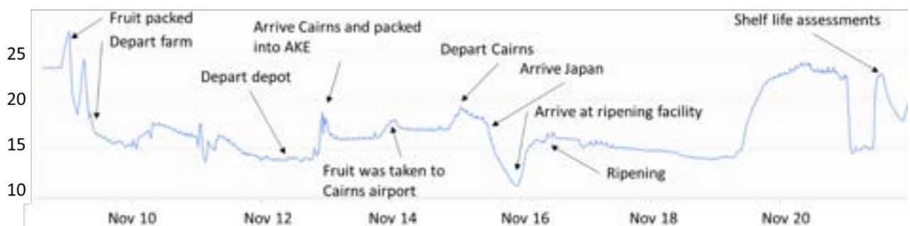
Figure 11. Changes in air temperatures within a box of Ecoganic® bananas from packing at a north Queensland farm, road freight to Cairns, air freight to Japan, ripening, through to display at a wholesale market. Data are representative of a box packed at layer 3 (centre) in an AKE air freight container.
