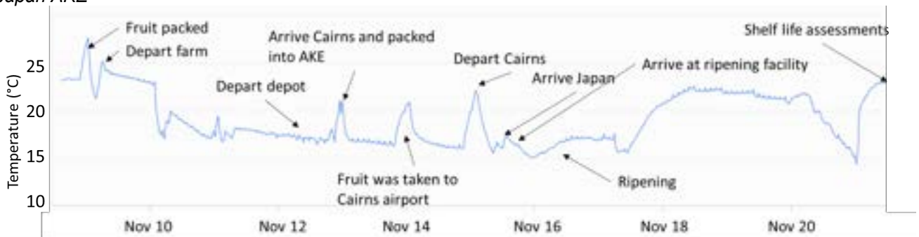
Figure 10. Changes in air temperatures within a box of Ecoganic® bananas from packing at a north Queensland farm, road freight to Cairns, air freight to Japan, ripening, through to display at a wholesale market. Data are representative of a box packed at layer 1 (base) in an AKE air freight container.
