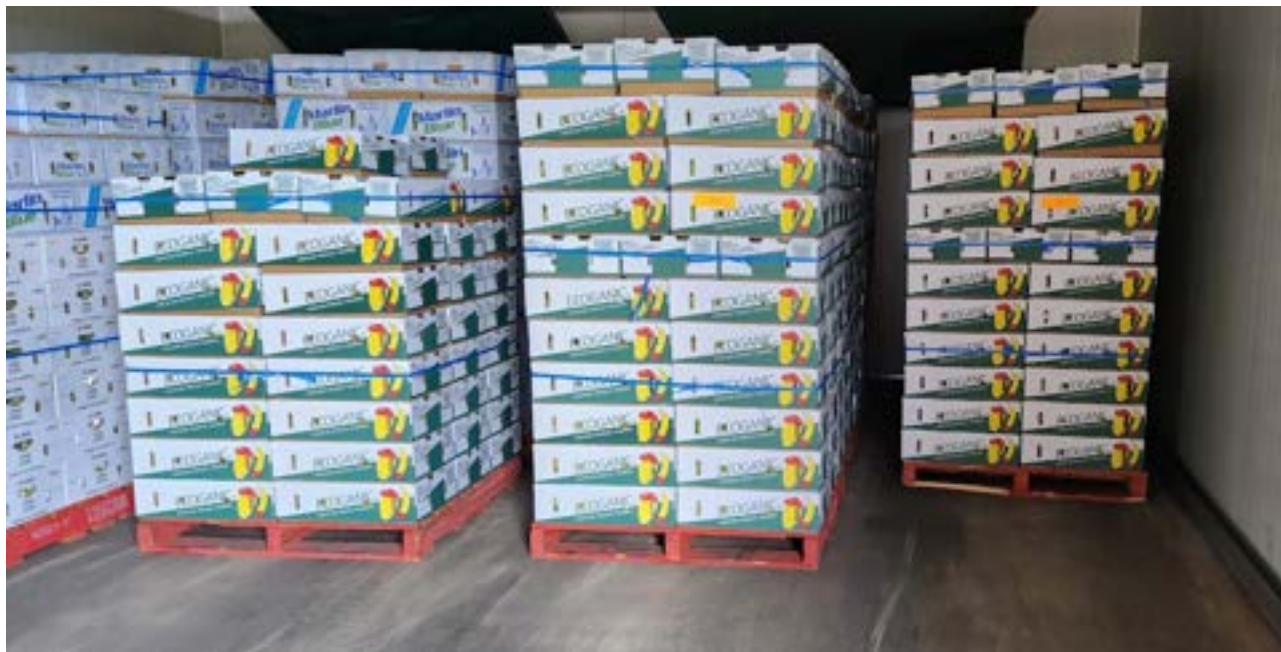
Figure 1. Photo of palletised boxes of bananas undergoing regular room cooling. Note spacing between pallets and alignment of box vent openings to aid cooling of fruit.
