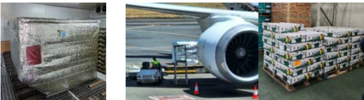
Figure 2. Photographs showing the layer of insulation applied to the AKE container (left), loading of the AKE onto the airplane (centre) and boxes of Ecoganic® bananas in storage at the ripener in Japan (right).
