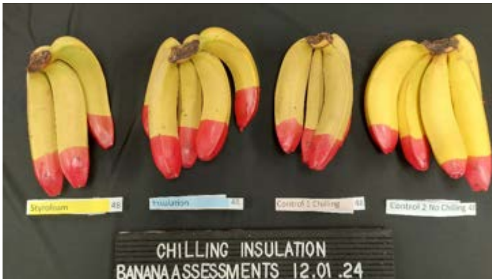
Figure 6. Styrofoam, insulation, chilled control and optimum storage control 2 during 5°C for 48 hours.
