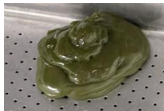
Figure 19: 5% Leaf protein product coming out of the extruder
