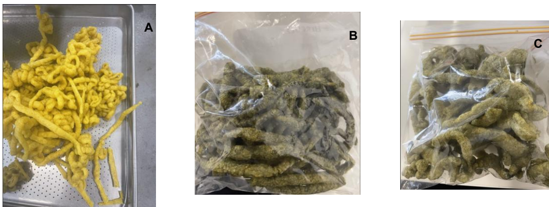
Figure 21: Extruded corn grits (A) and extruded leaf protein mixed with corn grits with high moisture (B) and after extruder was blocked (C)
