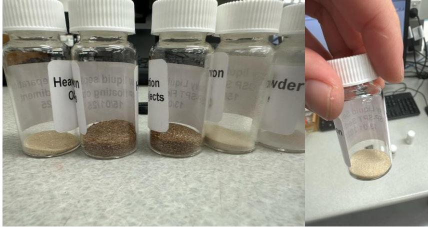
Figure 1. Separated molluscan shell fractions post-heavy liquid separation using sodium polytungstate (SPT).
