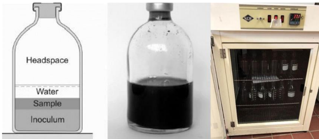
Figure 4 Example of batch biochemical methane potential assay (Left) and stored in a temperature-controlled incubator during testing (right)
